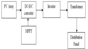
Fig.1.Block diagram of existing system
