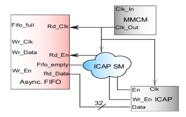
Figure 5: Block Diagram of ICAP controller.
