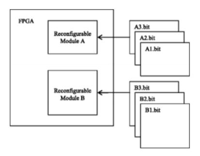
Figure 3: Multiple bit streams of Reconfigurable module
