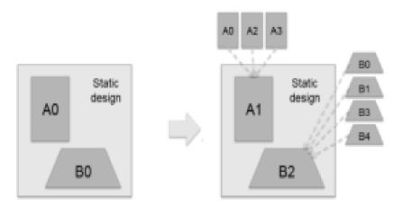
Figure 2: Difference between full and partial reconfiguration.
