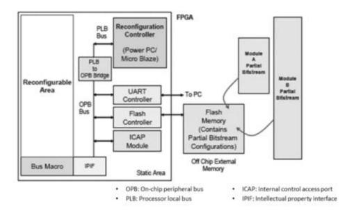
Figure 4: Block diagram of Dynamic Partial reconfiguration
