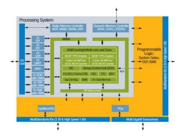
Figure 6: Implementation model of ZYNQ 7000 SoC.
