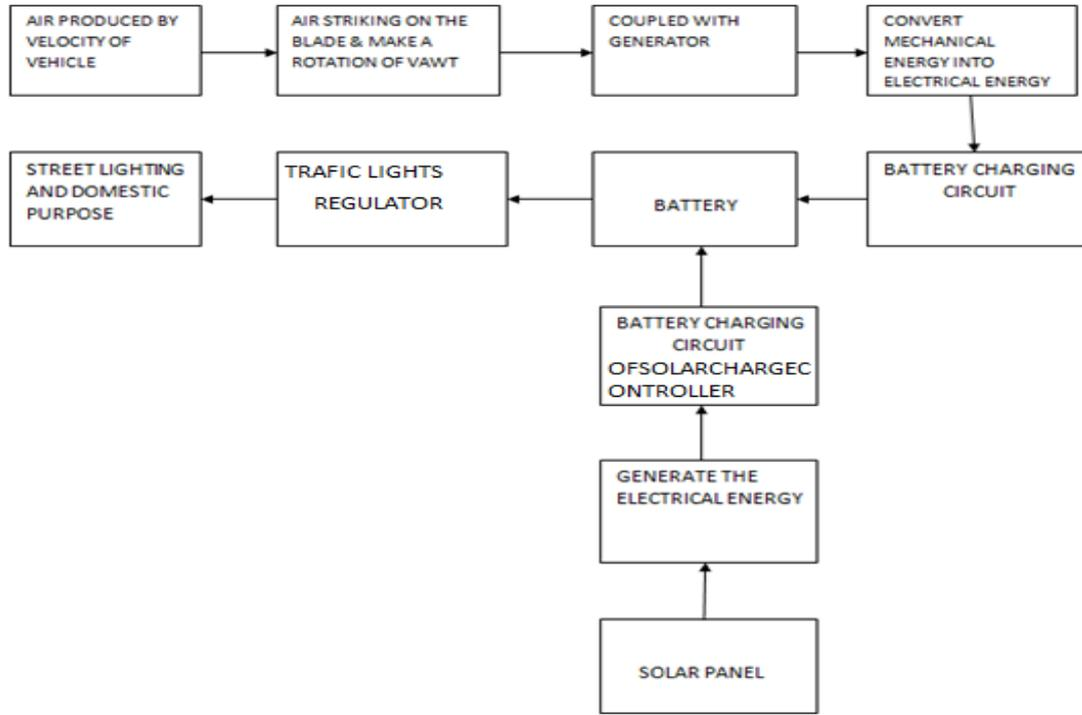
Fig. 7 Block diagram of working principle.
