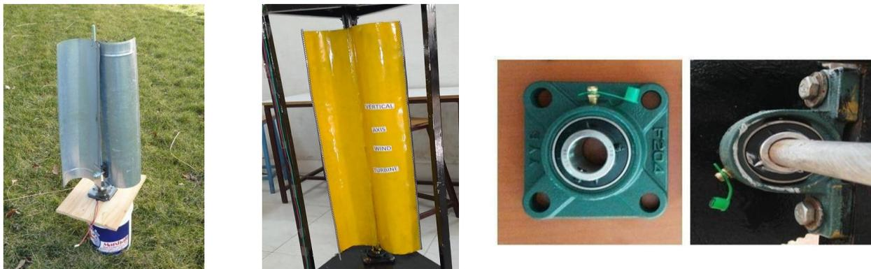
Fig 8 Turbine blades and shaft and bearings
