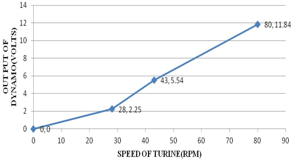
Fig. 9 Graph on output of dynamo Vs speed of turbine
