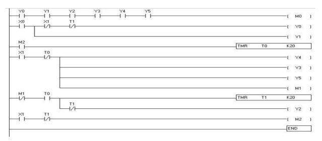
Fig 6 PLC ladder diagram for automatic bottle filling
