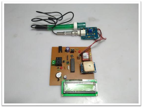
We implemented proposed system for detection of polluted water. We collected various results for different values of pH under different scenarios i.e. by using different types of water samples (neutral, acidic and basic). For neutral water we get pH=7, for acidic and basic water we get pH values less than and greater than 7 respectively. Depending upon the nature of water pH values are displayed on LCD.
