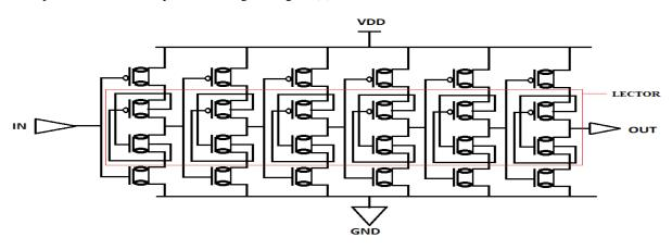
Figure 4: CNT Transistor based Three Stage Delay Line Circuit applying Lector Technique
