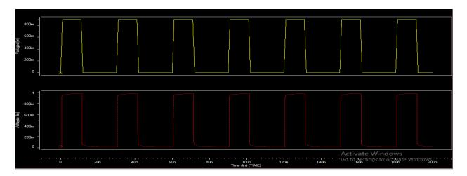
Figure 6: Waveform of Three Stages CNTFET based Delay Line with Lector Technique
