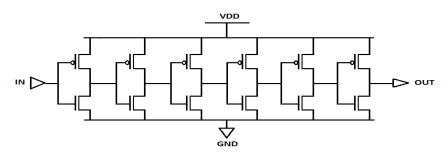
Figure 1: Three Stage Delay Line using CMOS Technology
