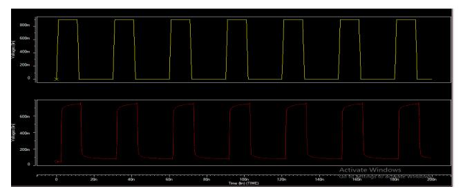
Figure 5: Waveform of Three Stage CMOS based Delay Line using Lector Technique
