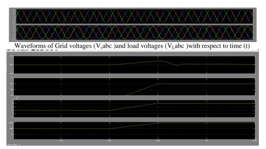
DC- link voltage( $V_{dc}$ ), solar PV array current( $I_{pv}$ ), PV array power ( $P_{pv}$ )in KW and Solar irradiation (G) in W/m<sup>2</sup> with time in sec.
