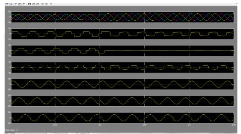
$\begin{array}{l} \mbox{Grid currents(} i_{sabc} \mbox{ ), Load currents(} i_{Labc} \mbox{ ), Shunt compensator currents (} i_{SHabc} \mbox{ ), with time (t ) in sec.} \\ \mbox{Fig.7 Performance of PV-UPQC during Load Unbalance Condition} \end{array}$
