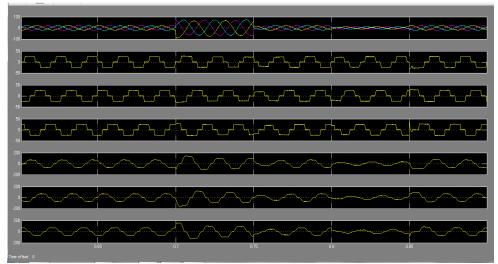
Grid currents(  $i_{sabc}$  ), Load currents(  $i_{Labc}$  ) Shunt compensator currents ( $i_{SHabc}$  ) with time (t )in sec
