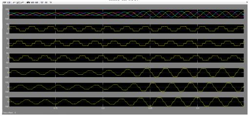
$\begin{array}{l} \mbox{Grid currents(} i_{sabc} \mbox{ ), Load currents(} i_{Labc} \mbox{ ), Shunt compensator currents (} i_{SHabc} \mbox{ ), with time (t ) in sec.} \\ \mbox{Fig. 8 Performance of PV-UPQC at Varying Irradiation Condition} \end{array}$
