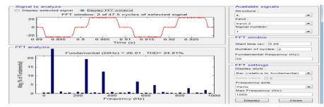
Fig.9 Load current Harmonic Spectrum and THD
