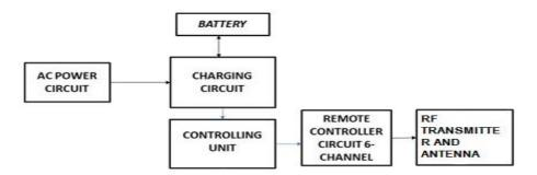
Fig 2: Transmitting part block diagram
