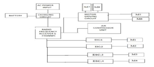
Fig 3: Receiving part block diagram
