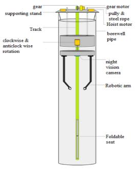
Fig 2: Rescue device setup
