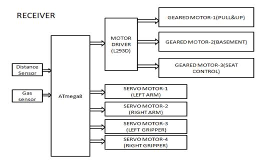
Fig 6: Receiver module
