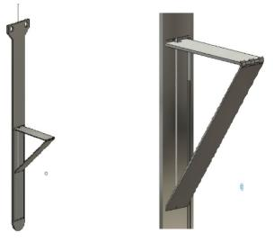
Fig 4: The supporting foldable arm
