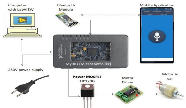
FIGURE 4: SCHEMATIC DIAGRAM OF SPEECH RECOGNISING CAR USING LabVIEW
