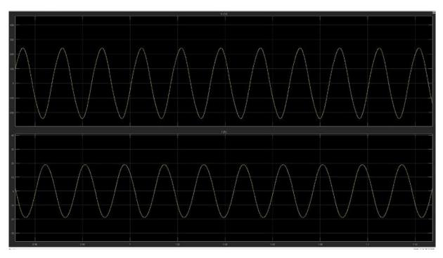
Output waveforms (a) CSI output current waveform and (b) grid voltage and grid current waveform
