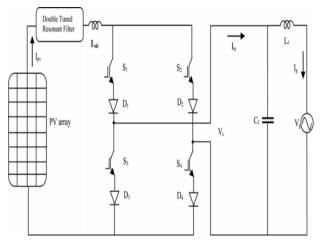
FIG1. Single phase grid connected CSI.
