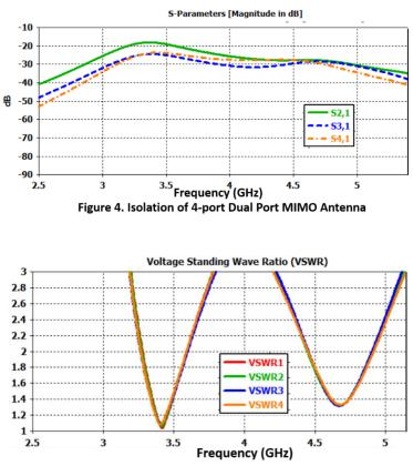
Figure 5. VSWR of the 4-port Dual Port MIMO Antenna
