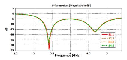
Figure 3. Reflection coefficient of 4-port Dual Band MIMO antenna
