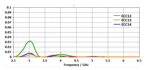
Figure 9. ECC of the 4-port Dual Band MIMO Antenna
