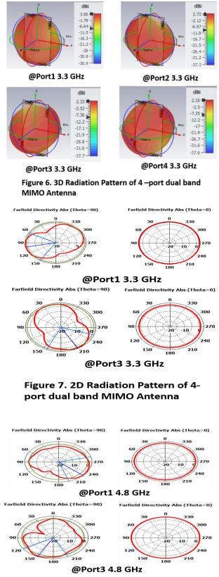
Figure 8. 2D Radiation Pattern of 4-port Dual band MIMO Antenna
