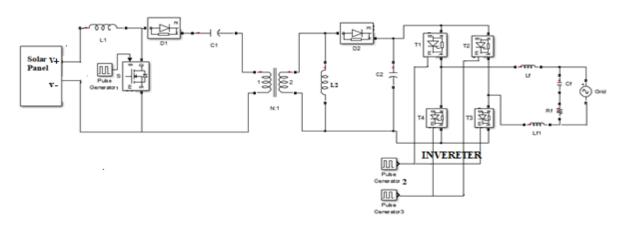
Fig.5. Proposed System Circuit Diagram
