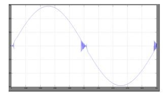
Fig .9.Inverter Output Voltage without Filter
