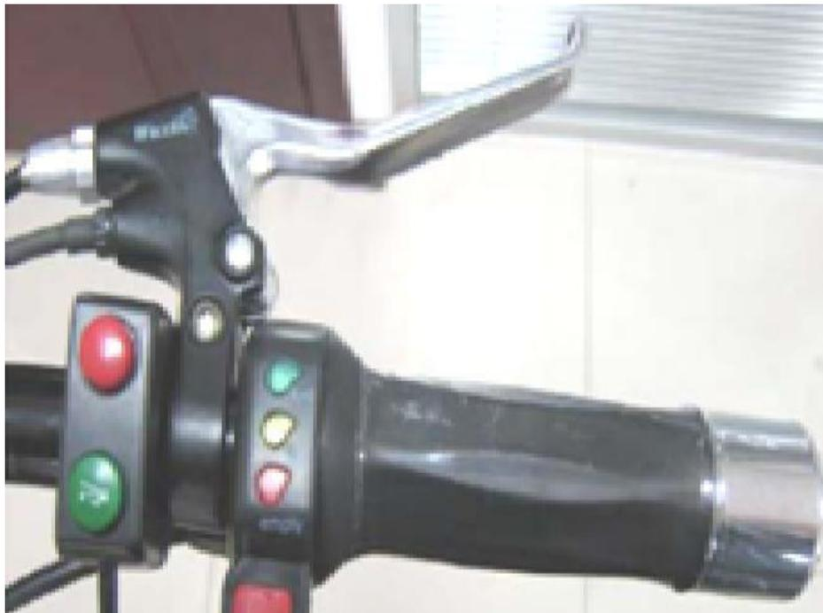
Fig 3 – Throttle / Accelerator
