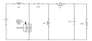
LUO is similar to a traditional <u>buck-boost converter</u>, but has advantages of having non-inverted output (the output voltage is of the same polarity as the input voltage), the primary means of coupling energy from the input to the output is via a series capacitor, and true shutdown mode.
