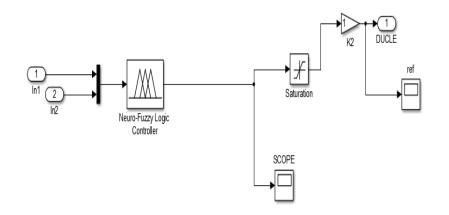
Fig.(d).simulink model of ANFIS controller
