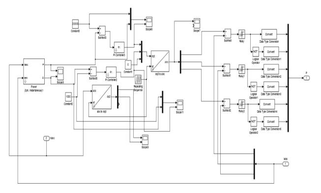
Fig.(e). Simulink model of PWM circuit for inverter
