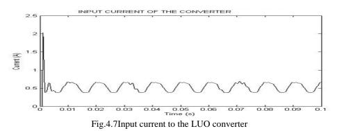
The above fig shows the input current given to the converter.
