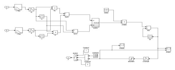
Fig.(c).Simulink model of PWM circuit for LUO-Converter
