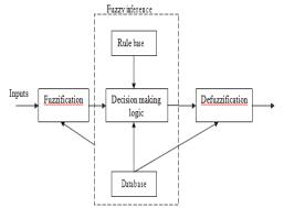
Fig2.2 Block Diagram of Fuzzy logic control
