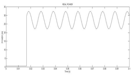
Fig.(a) Real power waveform of inverter
