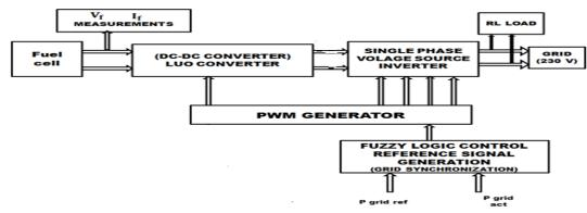
Fig.3.1Proposed system block diagram
