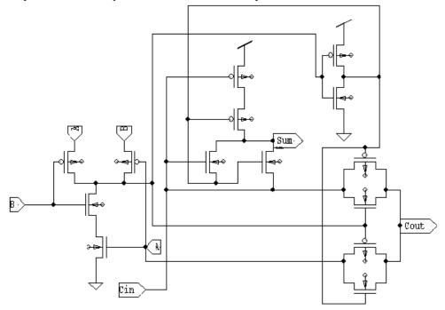
Fig 1: Circuit Diagram of Improved 14 T full adder
