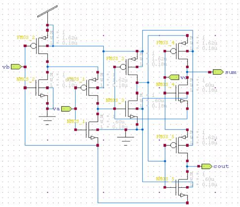
Fig 2: Schematic Diagram of GDI Adder
