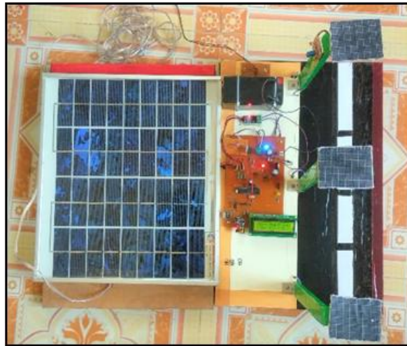
Fig.4.4 Street Light Is Off Condition In Day Timing
