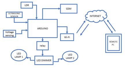
Figure 3.1 Project Block Diagram
