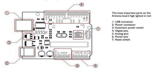
Figure 4.1. Arduino Pin Diagram
