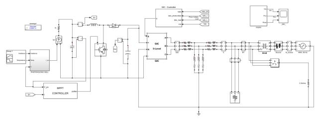
Fig.12.Simulink Diagram of the Grid Connected Photovoltaic System
