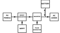
Fig.1. PV System Connected in Standalone Mode
