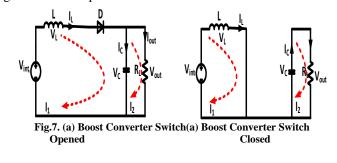
When the switch is 'OFF',  $V_L = V_{int} - V_{out}$
