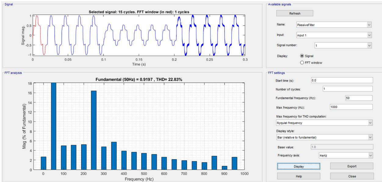
Fig.9 Harmonics distortion without DVR
