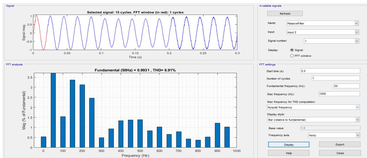
Fig.10 Reduction of Harmonics using Passive Filter based DVR
