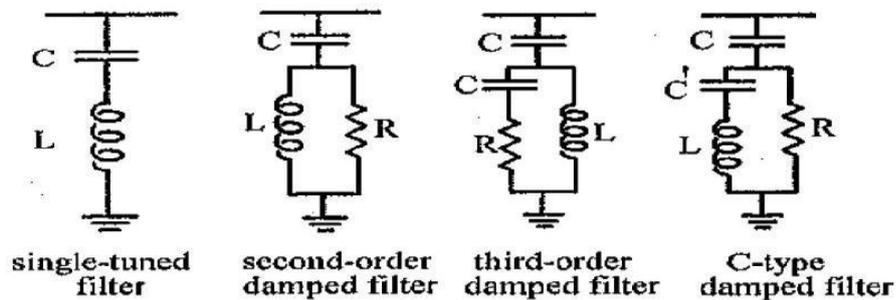
Fig.4 Shunt Passive filters
