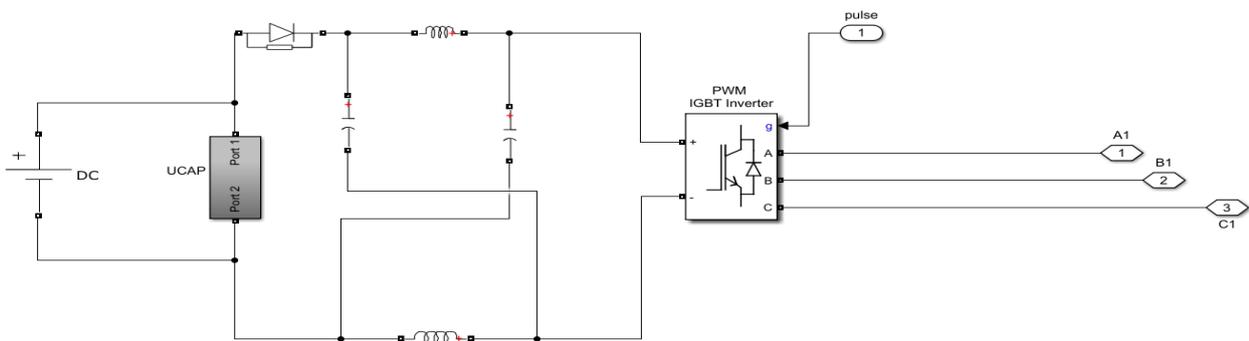
Fig.6 Z Source inverter
