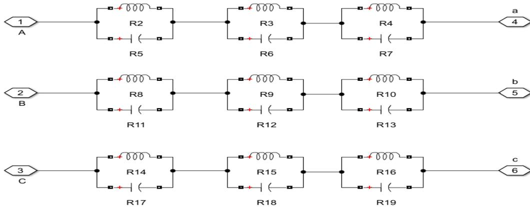
Fig.8 Model of Passive Filter
