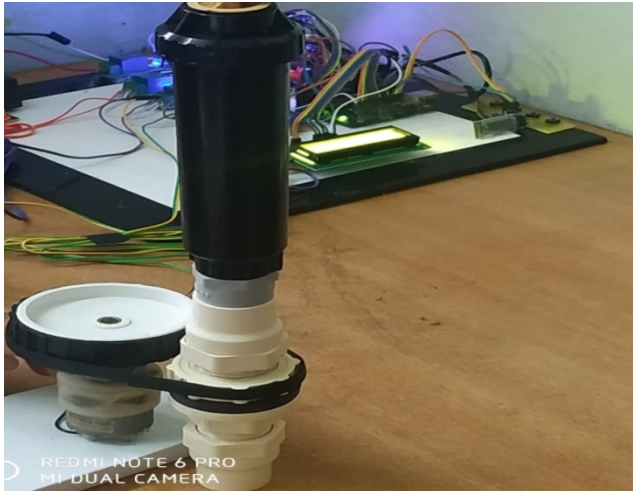
Figure 5: Sprinkler with DC motor
