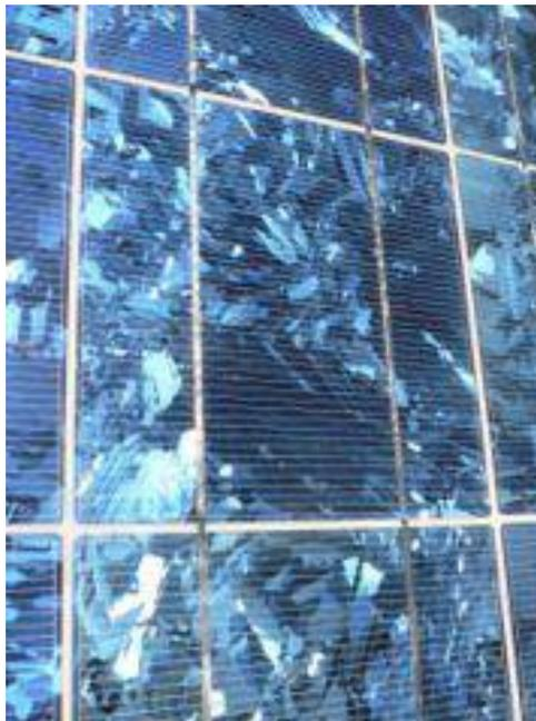
**Fig.1 Polycrystalline PV cells laminated to backing material in a PV module**
