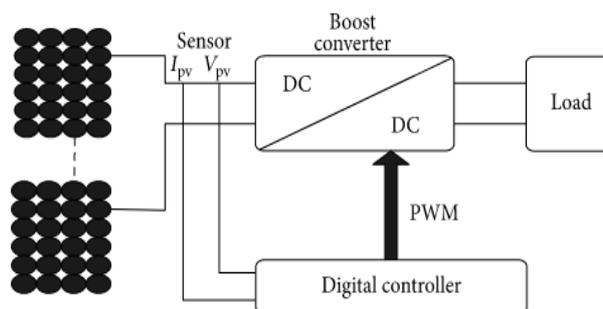
Fig.2 Block Diagram of PV Generation System
