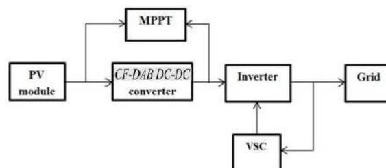
**Fig.3 Block diagram OF MPPT Techniques using DC-DC Boost Converter**
