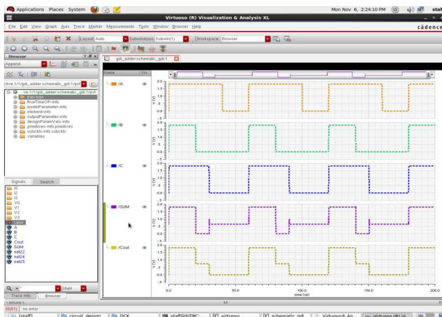
Fig -9: Output Waveform of GDI based Full Adder
