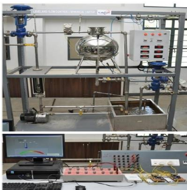
Figure.1 Experimental setup of spherical tank
