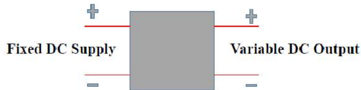
Fig 3: Basic Block diagram of DC- DC Converter
