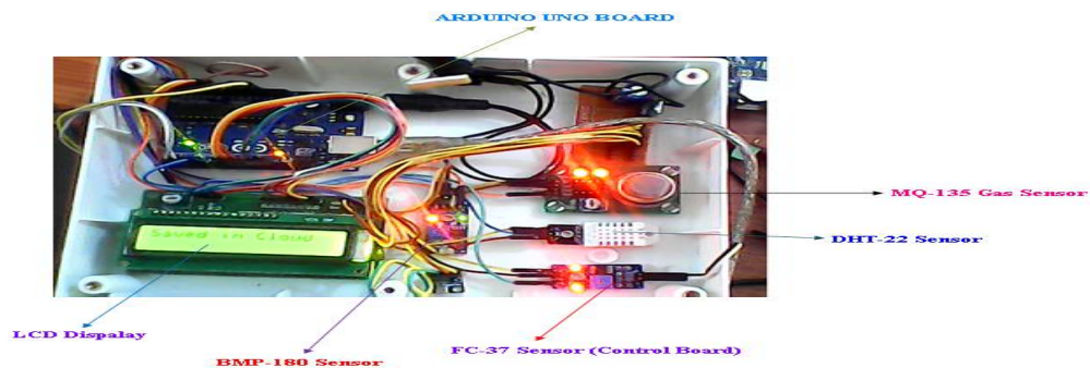
Figure 3: A Hardware setup for Thingspeak based Sensing and Monitoring System
