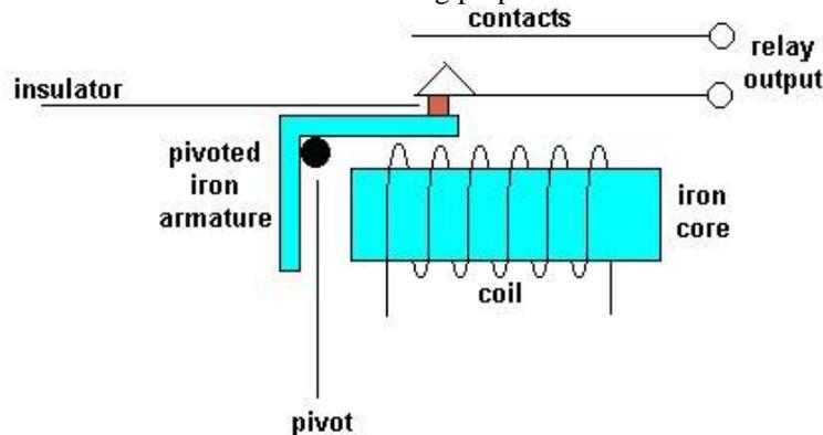
Fig7. Relay Circuit
