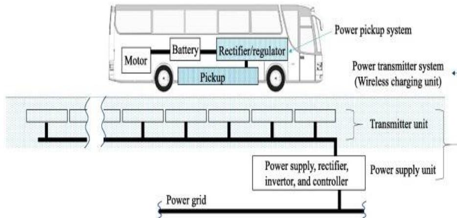
Poor coupling can result in poor transmission performance and low efficiency. Due to the large air gap between the primary and secondary windings, contactless transformers have large leakage inductances, small mutual inductance and low efficiency. Compared to direct contact charging, inductive charging efficiency is lower and resistive heating is.
