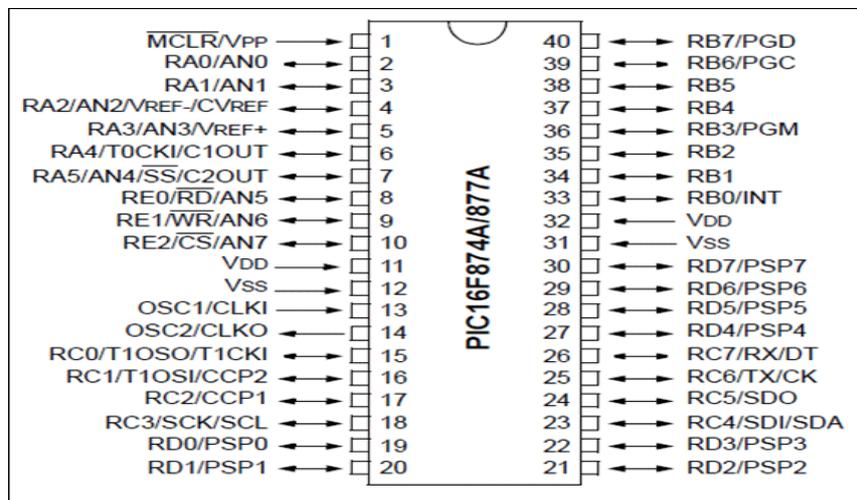
Fig4. Pin Diagram of PIC 16F877A
