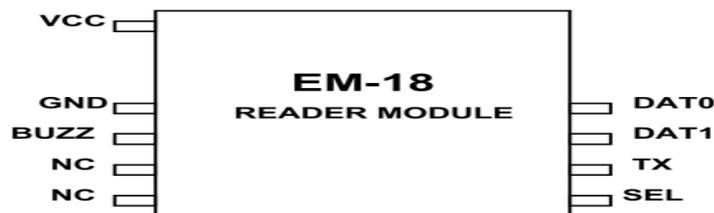
Fig5. EM 18 Reader module pin diagram
