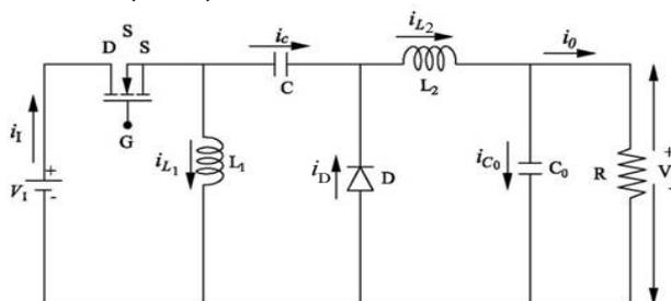
Fig. 1 Circuit Diagram of Positive Output Elementary Luo Converter
