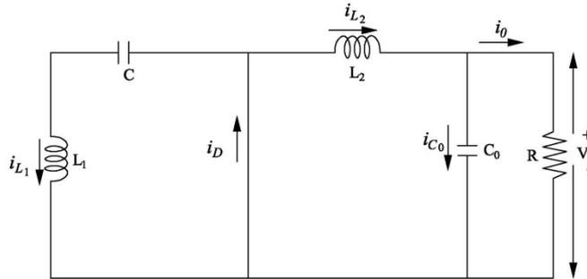
Fig. 3 Equivalent Circuit During Switch-OFF (Mode 2)
