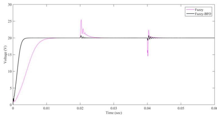
Fig.8 Output Responses under  $\pm 20\%$  Load Disturbances
