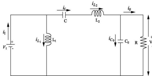
Fig. 2 Equivalent Circuit During Switch-ON (Mode 1)
