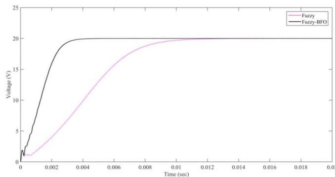
Fig. 6 Step Responses of Luo Converter with Fuzzy and BFOA-fuzzy Controllers
