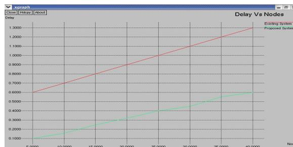
Fig. 2 presents the packet delay in both network coding-based and simple EOEERP protocols. In this point, we must recall that two packets are delivered to their respective destinations in each retransmission cycle . Hence, in order to be accurate, we compare the delay in EOEERP with the time required for two packets to be exchanged in EOEERP.As it can be observed, we can achieve significantly lower packet delay by applying network coding techniques.
