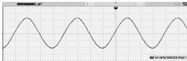
Fig.10 shows the sag condition voltage as visualized from the CRO.
