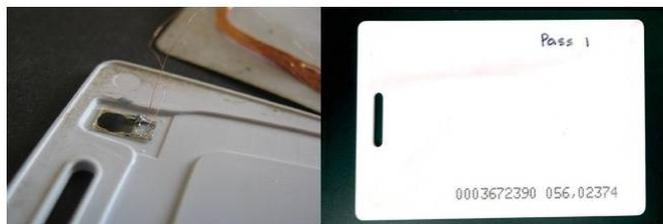
Fig 5: RFID tag (smart card)
