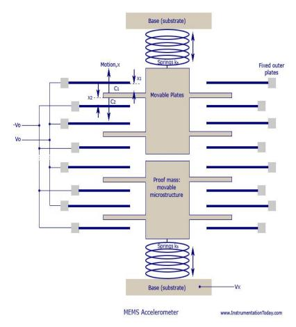
Fig 1. MEMS accelerometer sensor
