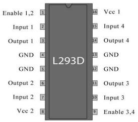
Fig 4 Pin diagram of L293D.
