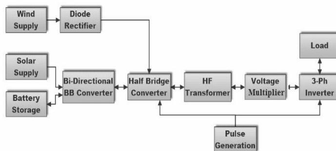
Fig. 1 Grid connected hybrid system with voltage multiplier for three phase applications.
