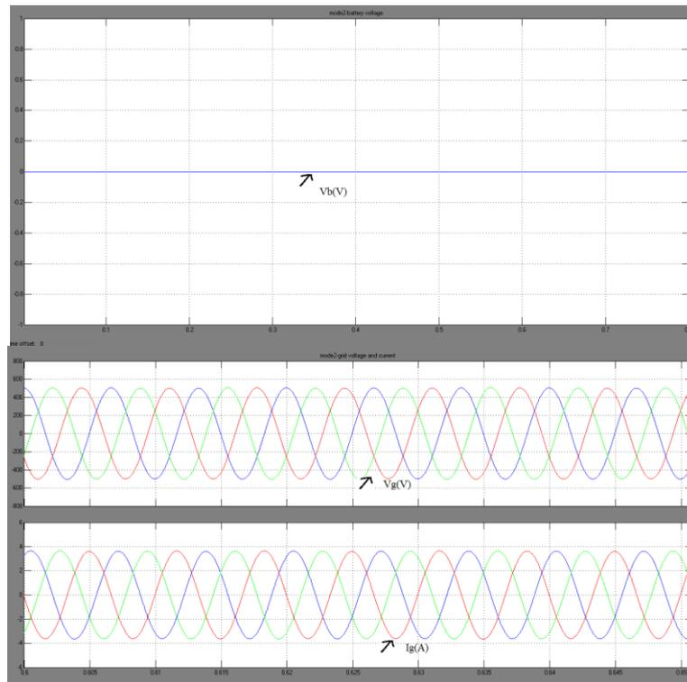
Fig.5. Response of the system in the absence of PV source while wind source continues to operate at MPPT
