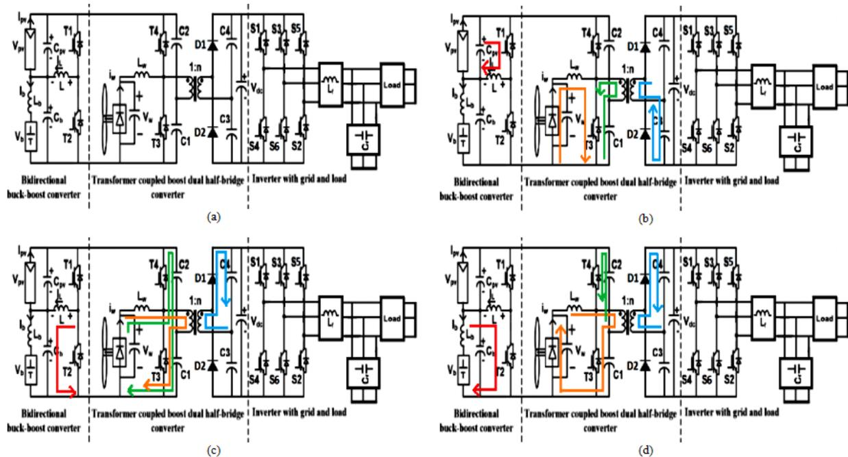
Fig. 2 operating modes of proposed hybrid grid connected transformer coupled bidirectional dc-dc converter for three phase domestic applications. (a) Proposed converter configuration. (b) Operation when switch T3 switch is turned ON. (c) Operation when T4 switch ON, charging the capacitor bank. (d) Operation when switch T4 ON, capacitor C2 discharging.
