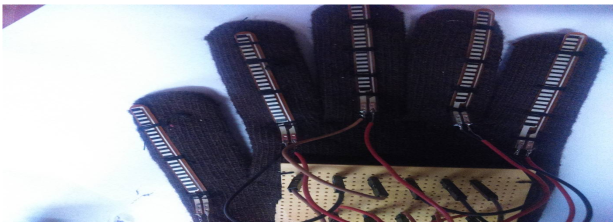
Fig:2 Flex sensors mounting
