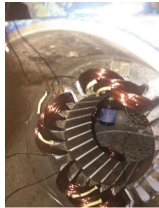
Fig. 10 b: With winding of Outer stator
