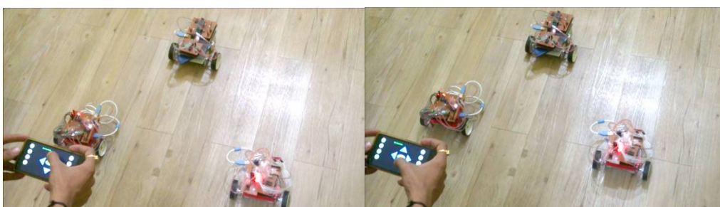
Fig.2 Forward Movement of robots When master is commanded to move forward, slaves move in same direction
