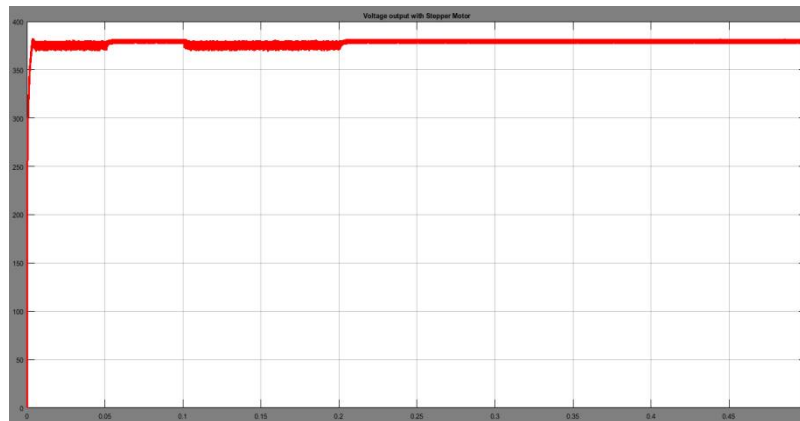
Fig. 10 Output voltage V_o of closed loop model TPC with ripple voltage content
