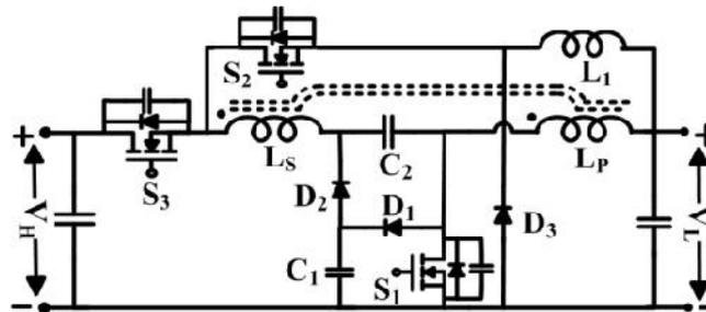
Fig.1 Proposed ZVS non-isolated bidirectional converter
