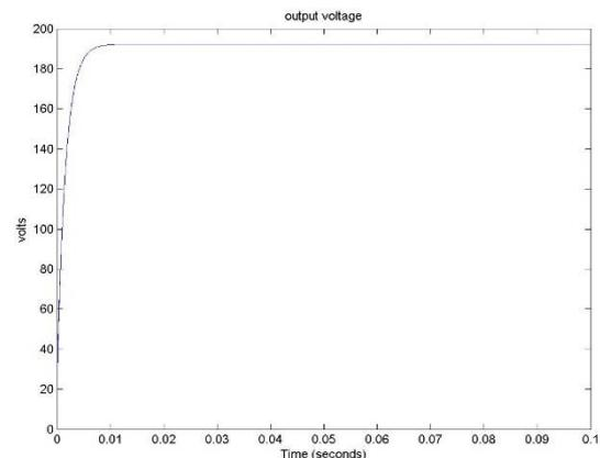
Fig. 4 Output voltage for boost mode of operation
