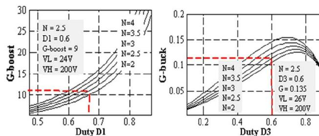
Fig.2 Gain duty ratio variation of converter
