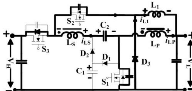
**Mode 5 ( $t_4 \sim t_5$ ):** The switch  $S_3$  turns ON under zero voltage switching (ZVS) condition. The capacitor  $C_1$  is charges through the clamped Diode  $D_1$ . The primary and secondary current starts increasing. At the end of this mode, the circuit starts repeating mode 1of the next cycle.
