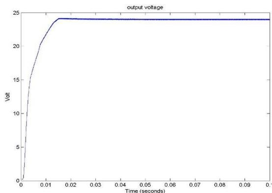
Fig. 3 Output voltage for buck mode of operation.
