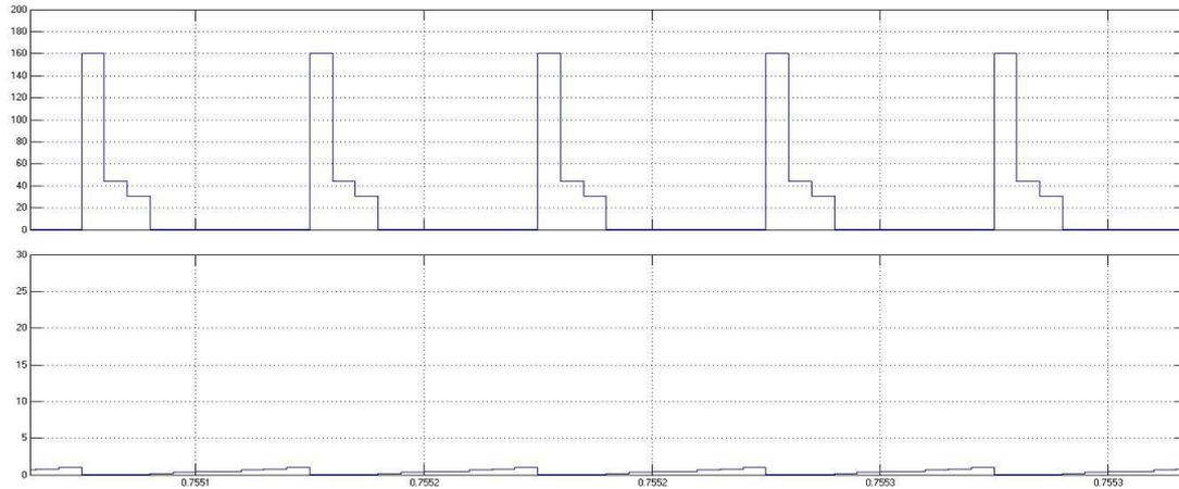
Fig.5 Zero voltage switching of main switch s2
