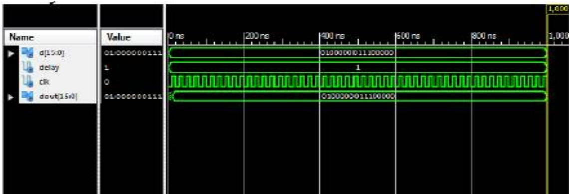
Fig 12: Xilinx ISE Simulation of Delay block
