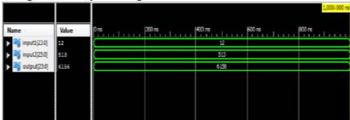
Fig 11: Xilinx ISE Simulation of Baugh Wooley Multiplier
