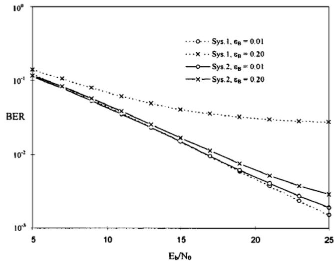
Fig. 3: BER Comparison for Urban Area Channel Model
