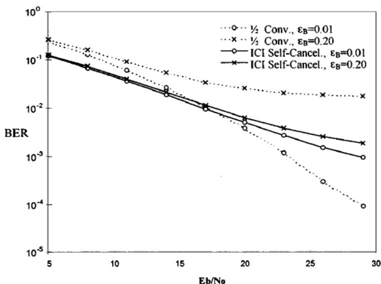
Fig. 5: BER of Error Correction Coding and ICI Self-Cancellation Scheme
