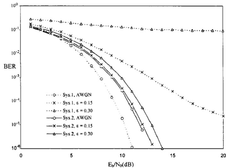
**Fig. 2: BER vs.  $E_b/N_0$  (dB) of Two Systems for Different  $\epsilon$  Values**
