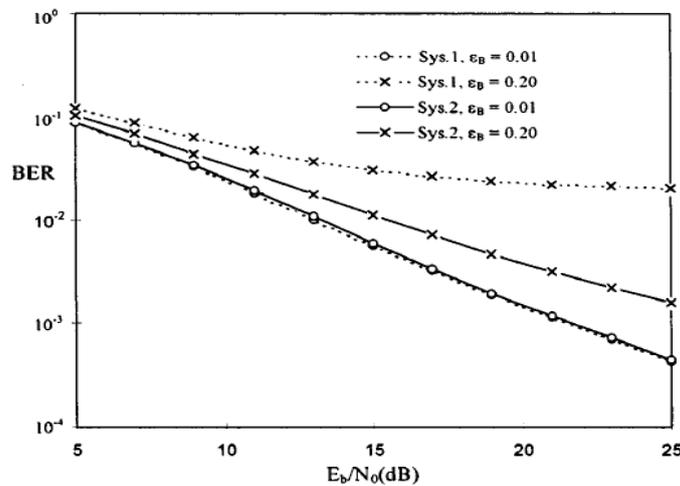
Fig. 4: BER Comparison for Rural Area Channel Model
