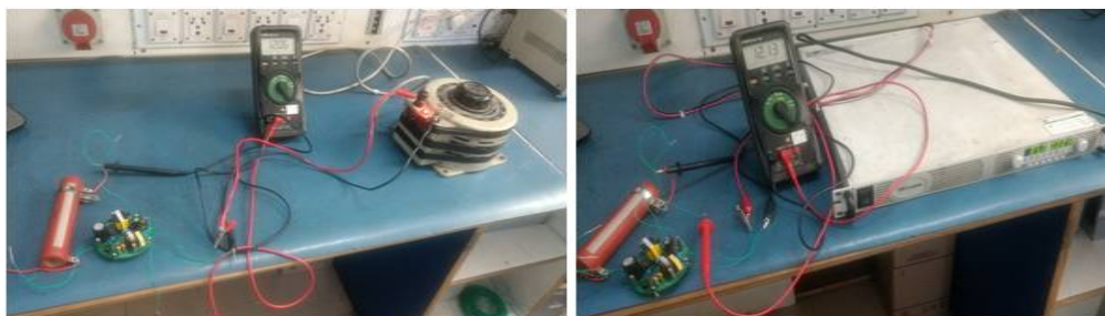
Fig.5 (a) Test setup of the proposed converter with AC input voltage, (b) DC input Voltage
