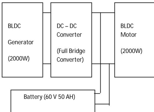
Fig. 4 System with Single Input DC-DC Converter (Topology 2) Converter (Topology 1)
