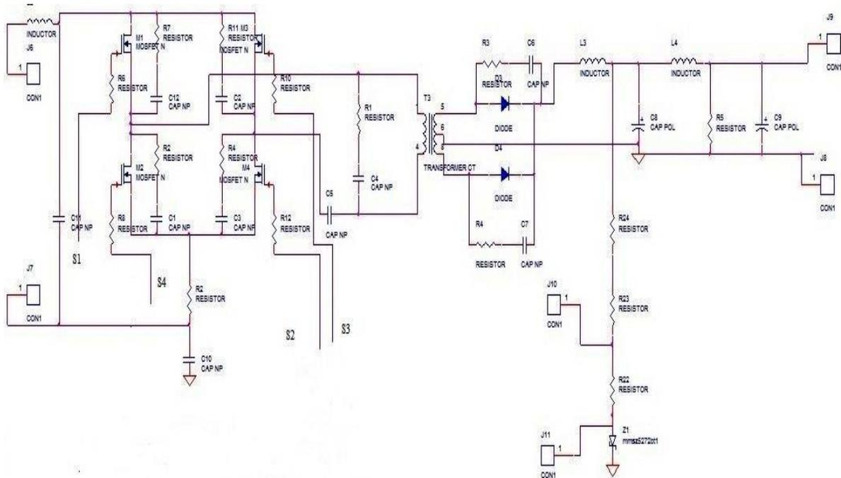
Fig. 16 Full Bridge DC-DC Converter
