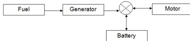
Fig. 2 Basic Block Diagram of Series Hybrid vehicle indicating power flow among the blocks
