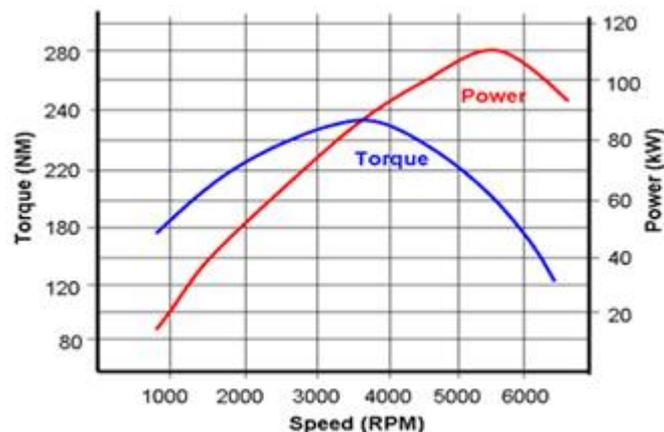
Fig. 1 Power and Torque graph of engine
