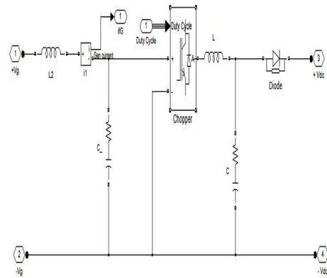
Fig 13 Components inside DC-DC Converter
