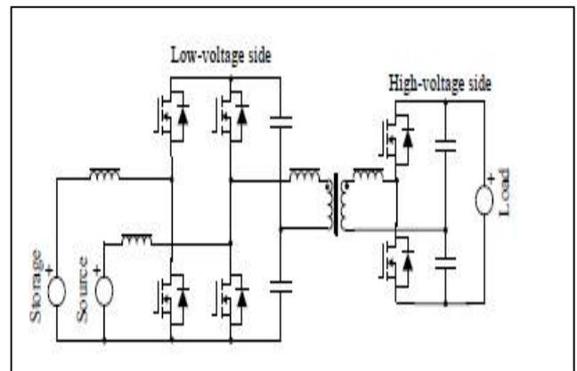
Fig. 3 Multi Input Multi Output DC-DC
