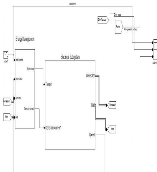
Fig. 7 MATLAB SIMULINK model showing basic blocks such as energy management and electrical subsystem
