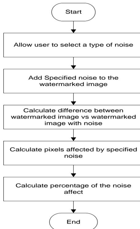
Fig 4: Flow chart of noise attack measurement.
