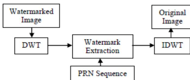
Fig 3: Block diagram of watermark extraction.
