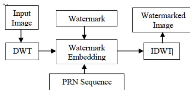
Fig 2: Block diagram of watermark embedding.
