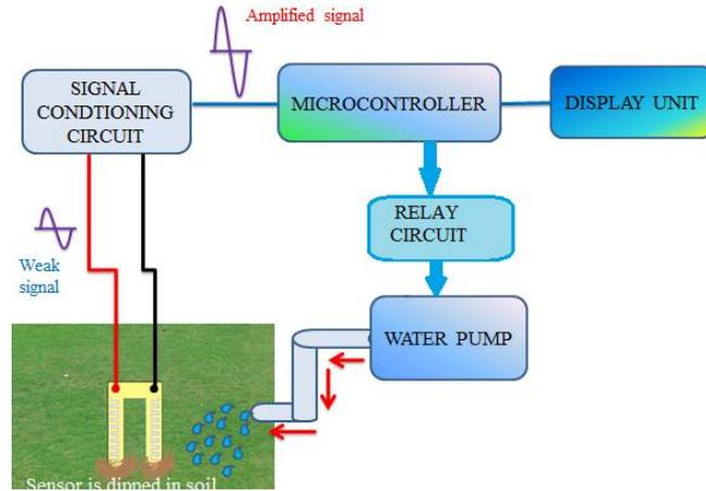
Fig.2. Block diagram irrigation system
