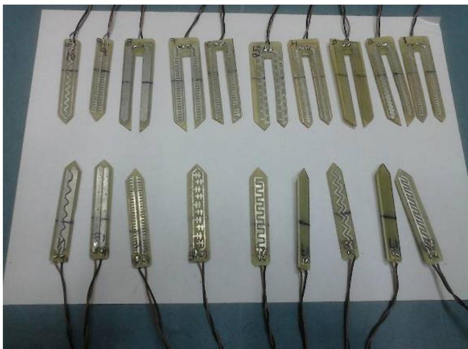
Fig.1 Lab made sensors with different patterns.
