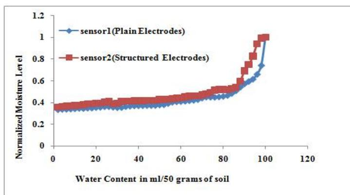
Fig.6: Normalized sensed value corresponding to water content in ml/50grams of soil in a container.
