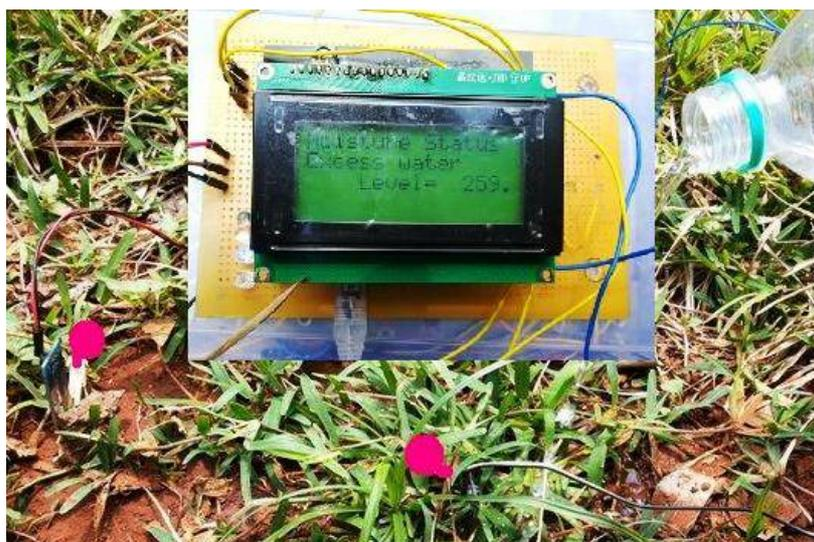
Fig.4: In a cropping field the moisture level is tested in dry area and the excess water area. Display shows the excess water level with one of the sensor.
