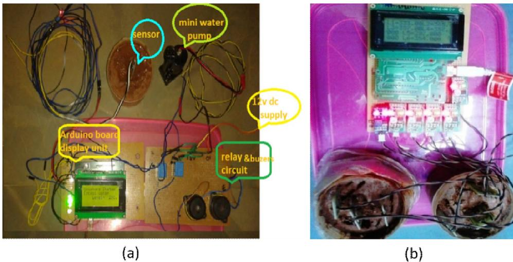
Fig.3 (a) Physical components diagram of automatic watering system. (b): Six sensors at a time are checking to make the sensitivity level
