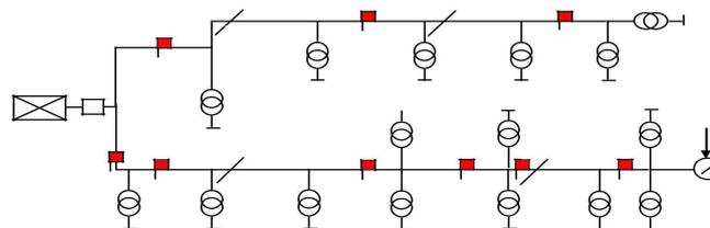
fig.1: Radial structure with FPIs
