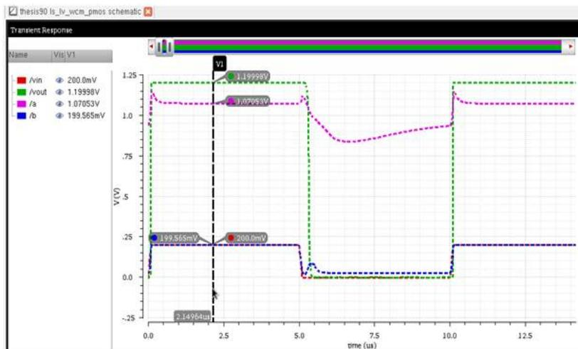
Fig. 7. Vin and Vout waveforms for 0.2 to 1.2 v conversion
