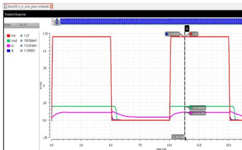
Fig. 8. Vin and Vout waveforms for 1.2 to 0.2v conversion
