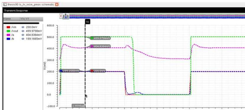
Fig. 4. Vin and Vout waveforms for 0.2 to 0.5v conversion
