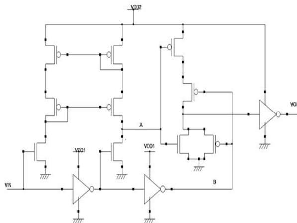
Fig. 1. MWCMHB level shifter.
