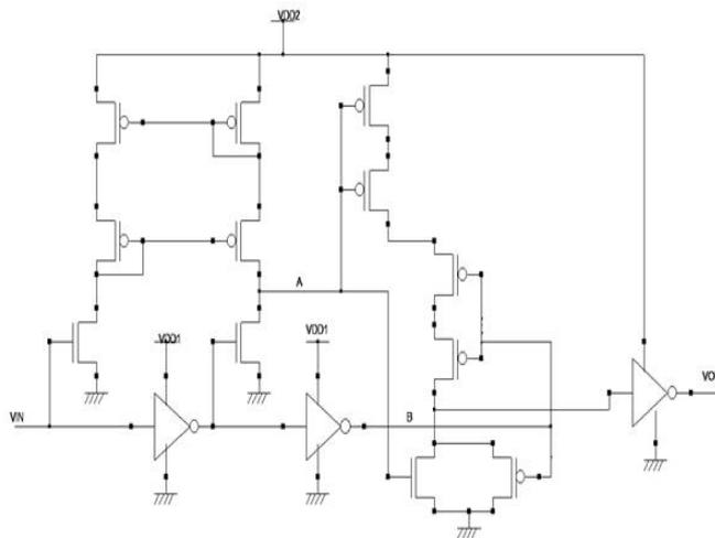
Fig. 2. MWCM based LS using stacking technique.
