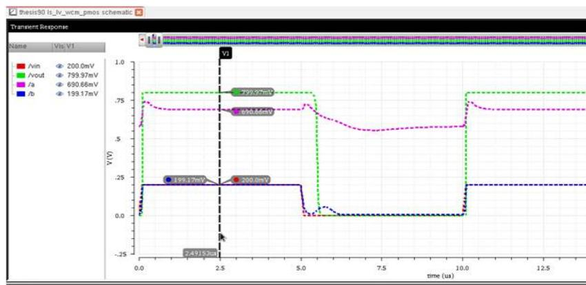
Fig. 5. Vin and Vout waveforms for 0.2 to 0.8v conversion
