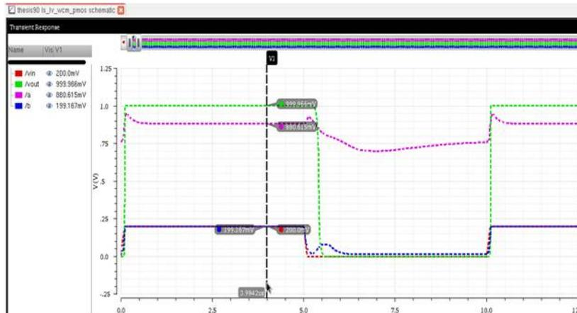
Fig. 6. Vin and Vout waveforms for 0.2 to 1v conversion
