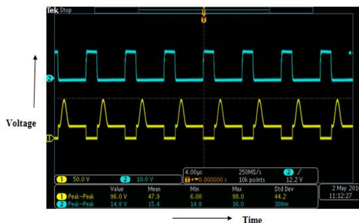
Fig 13: Gate and drain waveform of 15V/1A converter at 28V input voltage and full load condition.
