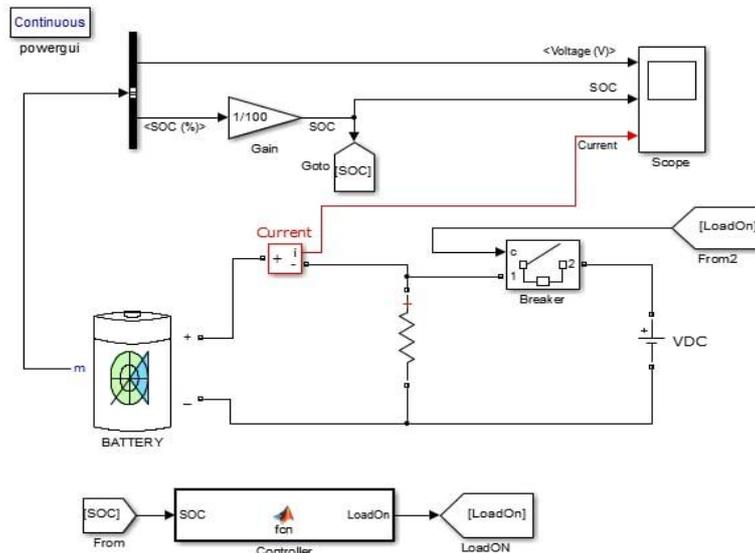
**Fig-5:** The simulation of the hybrid power source using MATLAB Simulink.
