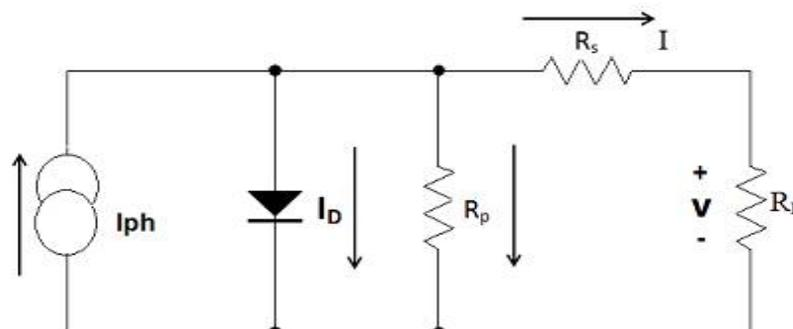
Fig.3. PV single diode model
