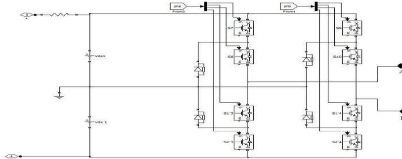
Fig.2. NPC Three level inverter model
