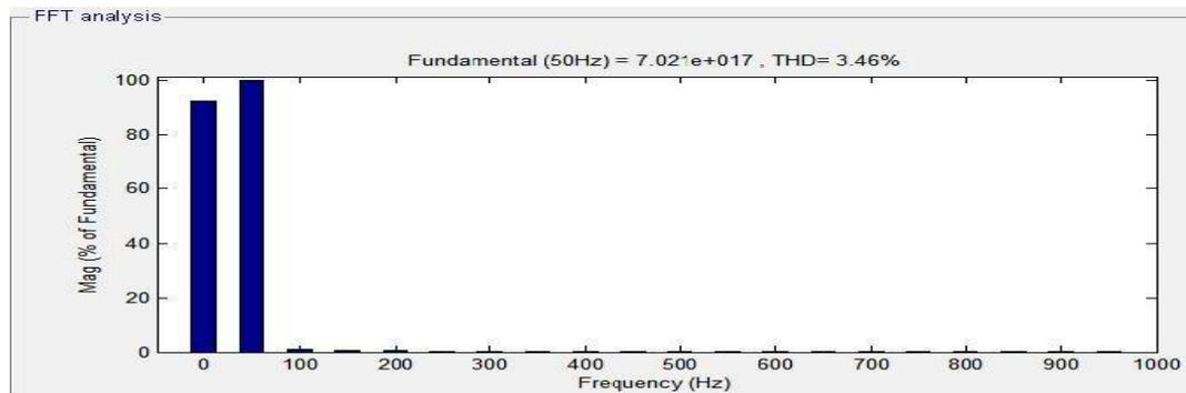
Fig.7. Total harmonic distortion of inverter current
