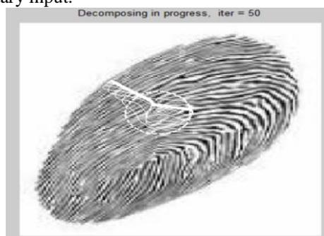
Fig. 2 Decomposing the image to find the minutiae points with 50 iterations.
